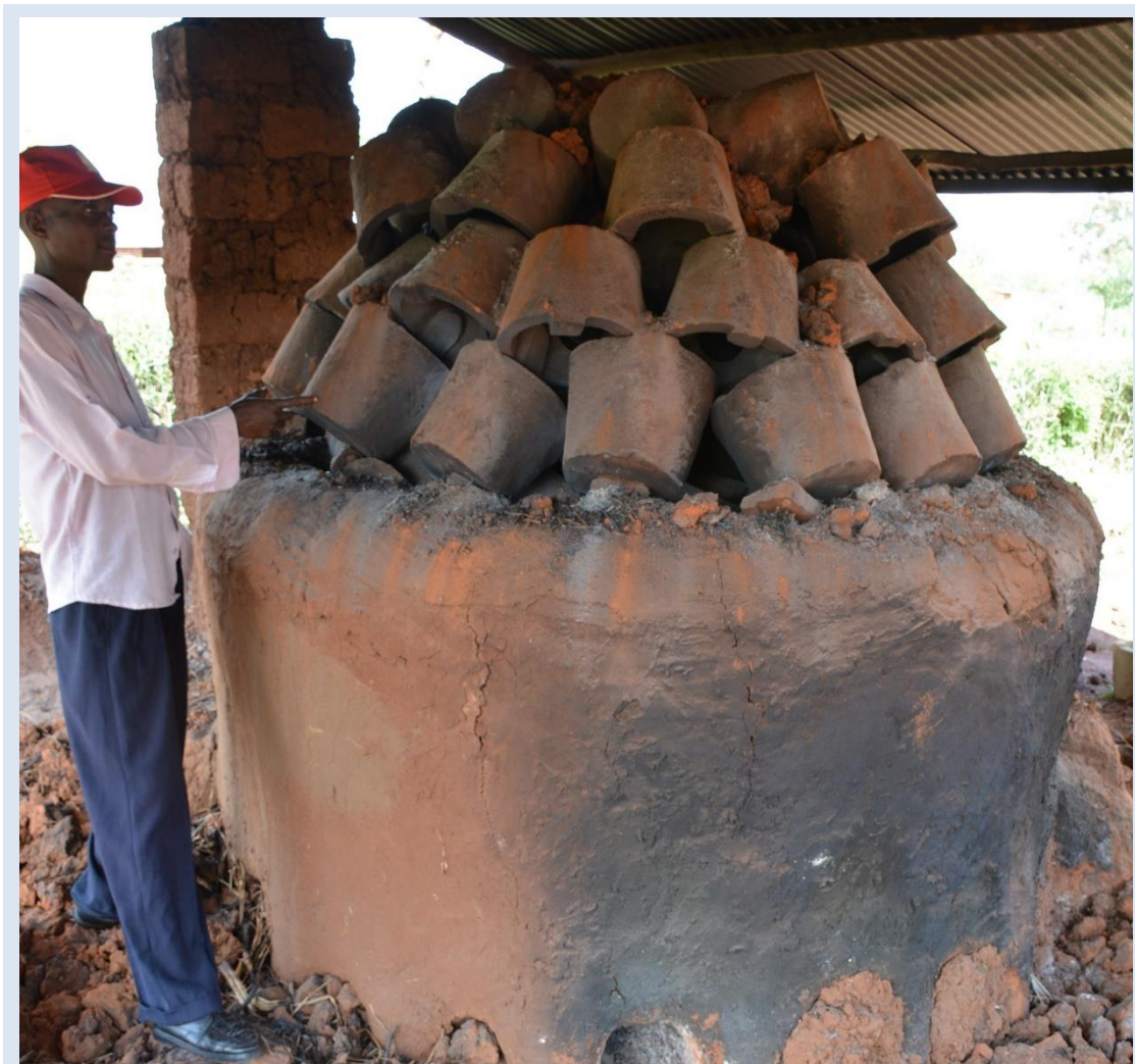
A kiln for firing stoves at a manufacturing cooperative in Rwanda.
