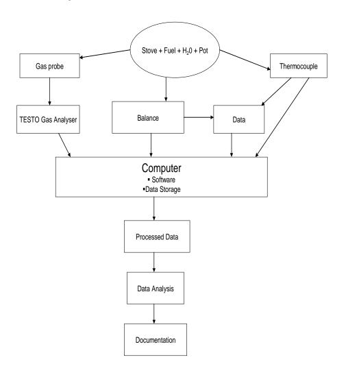
The heterogeneous testing procedure for thermal performance
