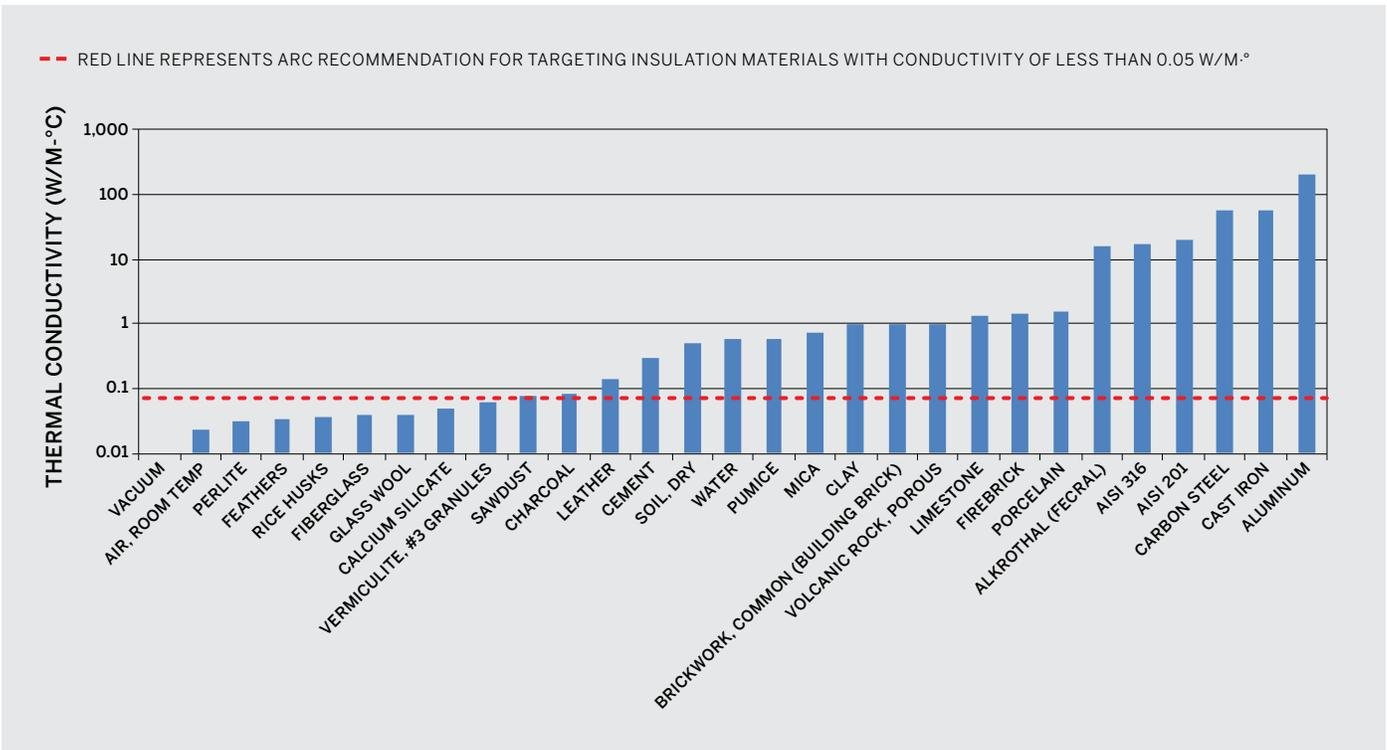
Increasing the thickness of the insulation layer decreases the amount of conduction heat transfer through the insulation. However, increasing the thickness also increases the external surface area and the radiative and convective losses on the exterior surface of the stove, so the insulation thickness and external surface area must be balanced.
