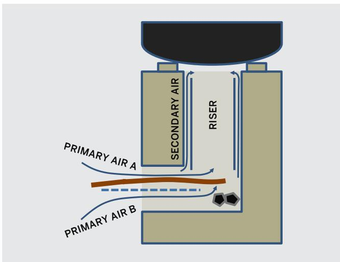
**FIGURE 10:** MODES OF AIR SUPPLY IN A FORCED-DRAFT GASIFIER COOKSTOVE
