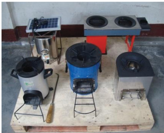
Fig. 1. Trial stoves, clockwise from top left: Eco Chula, Prakti, Envirofit, EcoZoom, and Greenway.
