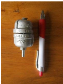
Figure 3: Traditional SUM Holder copyright of Kirk Smith's lab used in Mexico study
