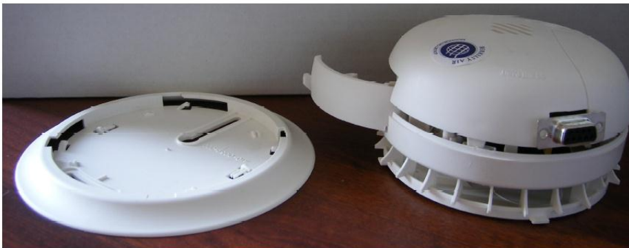
Figure 2: Space created by loosening the UCB PM lid from the base.
