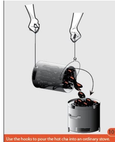
Use the hooks to pour the hot charcoal into an ordinary stove.
