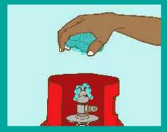
Use soapy water to check for gas leak, not naked flame.
