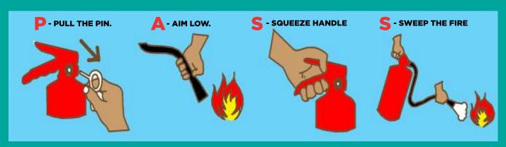
Hold extinguisher with nozzle pointing away from you and release locking mechanism.
