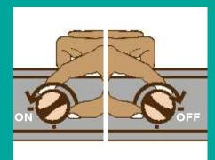
Turn on the burner by rotating the knob anti-clockwise, shut it off after use by turning the knob clockwise.
