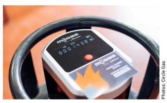
Circle Gas' proprietary smart meter, located directly on the LPG cylinder, reports gas consumption back to Circle Gas systems to support billing and the scheduling of replacement cylinders.
