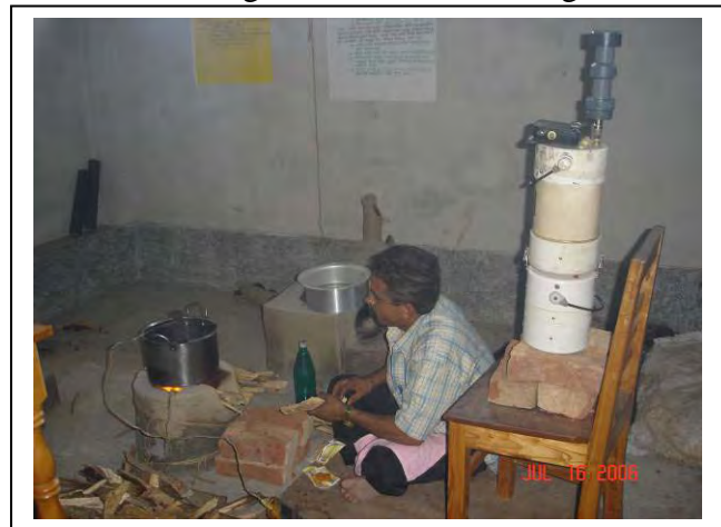
WBT simmer test in progress Photo credit: Winrock
