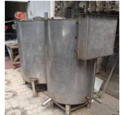
Steam boiler for tofu production
