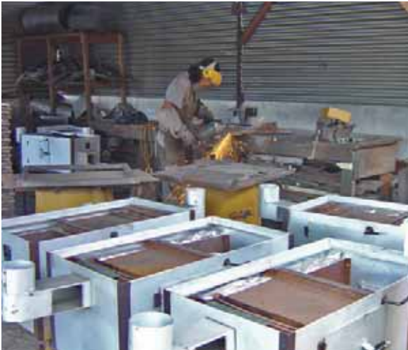
PHOTOGRAPH 7 Justa Ecostove being manufactured in Honduras by ADHESA
