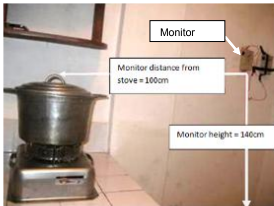
Figure 5.33: IAP monitoring installation
