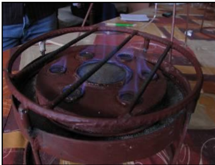
Figure 5.5: Top view of multiple burner stove
