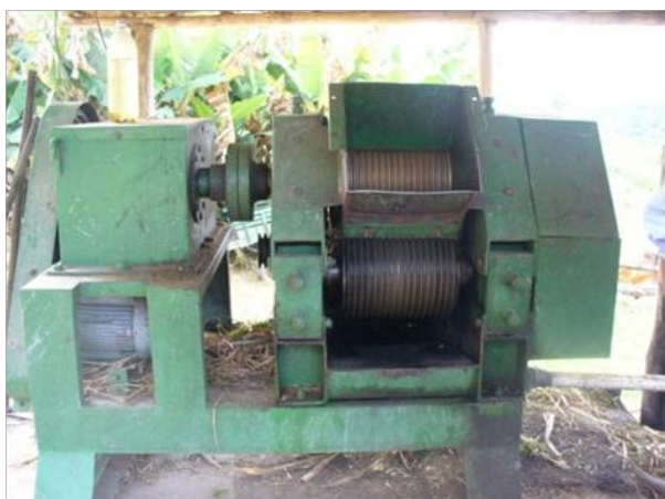
Figure 2.6 Sugar cane mill
