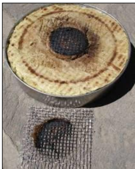
Figure 2.2: Ethanol laden with fusel oil. The top of the canister was removed for this photo (Gaia Association).
