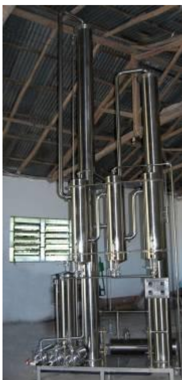
Distillation unit: 1000 litres per day
