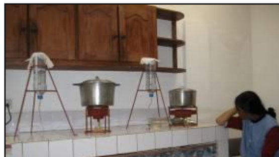
Figure 5.7: The single and multiple burner stoves during the water boiling tests
