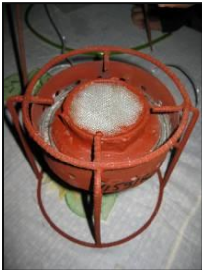
Figure 5.4: Top view of a single stove burner
