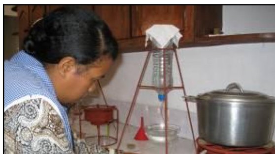
Figure 5.6: Regulating the fuel flow to the stove
