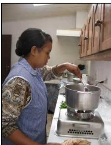
Figure 5.8 (left): CleanCook stove during CCT
