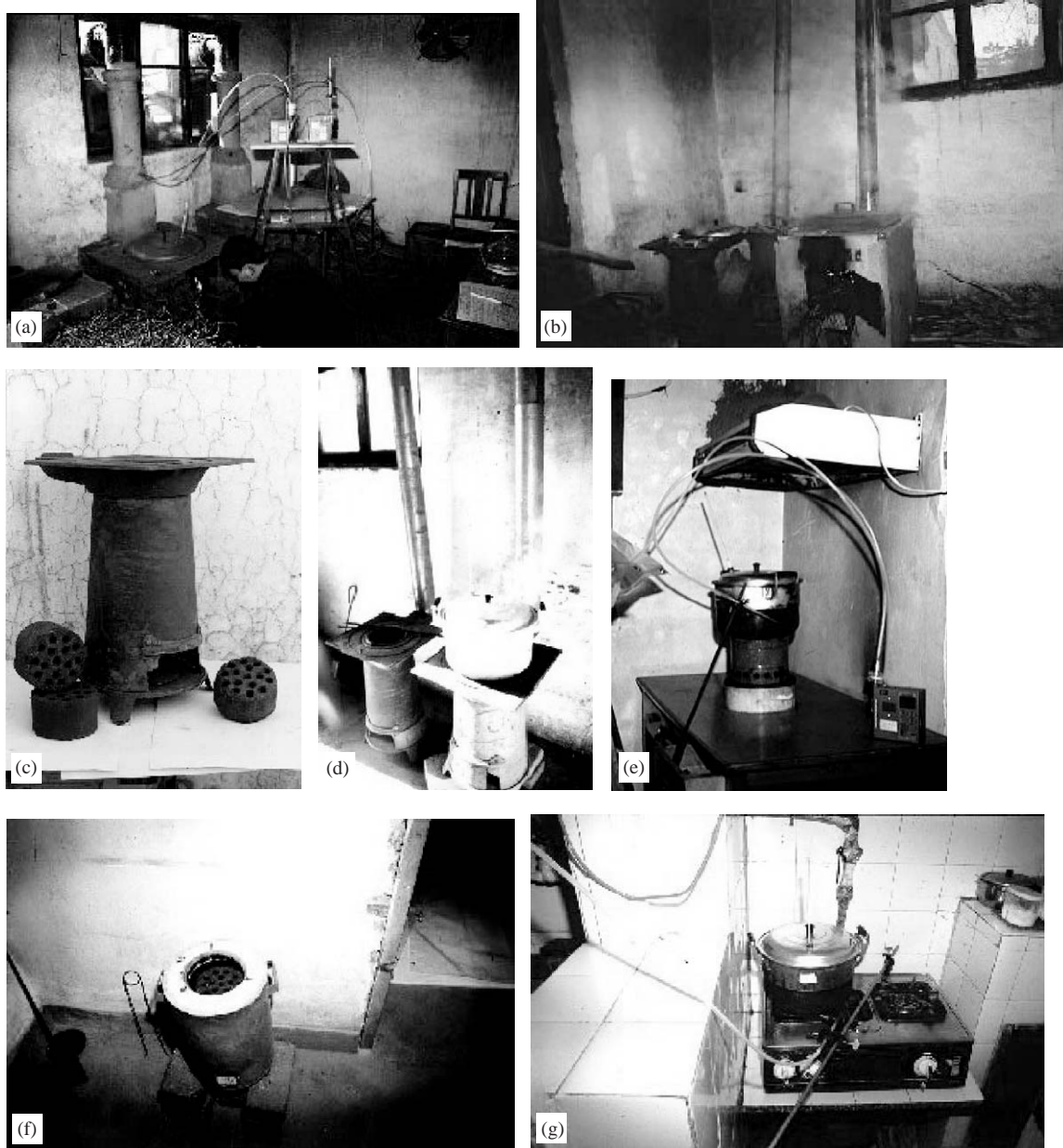
Fig. 1. Chinese Stoves (a) brick stoves, traditional (with the fire) and improved, both with a flue. Both types of stove can burn wood, crop residues, and unprocessed coal. (b) metal stove with flue (burning wood), (c) traditional metal coal stove without flue, beside the stove are honeycomb coal briquettes. (This type of stove can also burn coal briquettes.), (d) metal coal stoves with flue (both honeycomb coal and coal briquettes can be burnt in these stoves.), (e) Kerosene wick stove with sampling set-up, (f) improved metal coal stove without flue (designed for honeycomb coal briquettes), and (g) traditional gas stove.
