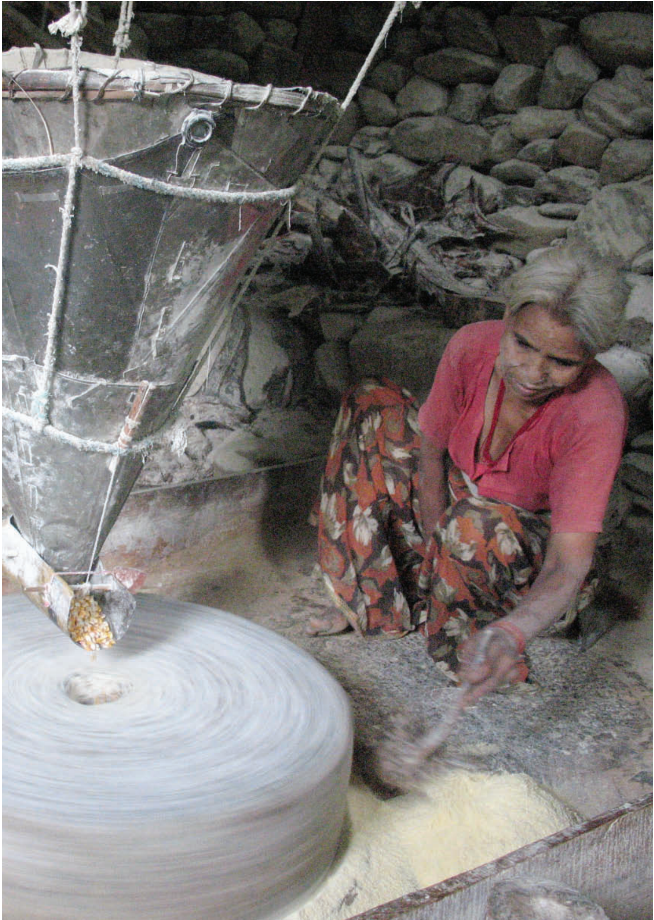
A woman operating a rice husker using an improved water mill. Project: IWM – Nepal.
