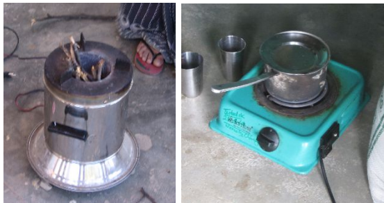
Figure 2. Two types of ICS: (Right) Forced-draft biomass ICS; (Left) Electric coil ICS.
