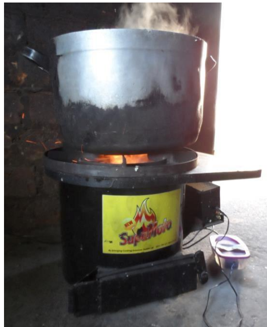
Figure 34: An institutional stove burning pellet fuel supplied by ECS in Zambia
