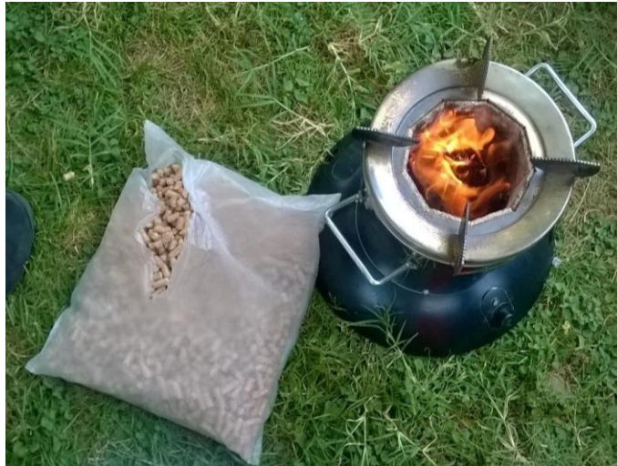
Figure 17: Pellet burning in the Philips gasifier stove
