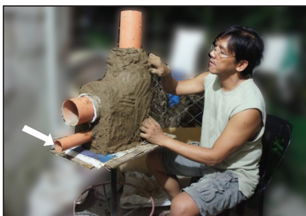
Modifying the stove design for easier ash removal
