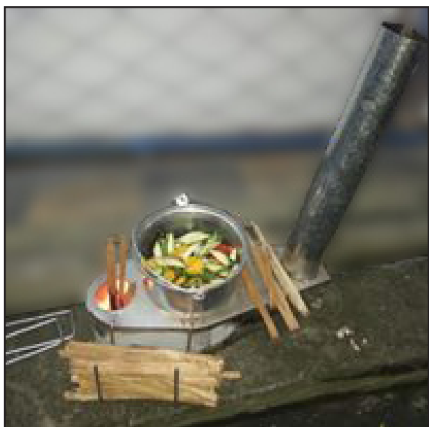
The vertical-fed biomass cookstove at work
