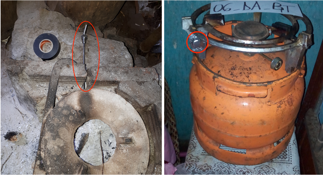
Figure 4: (Left) A stove fit with a K-type thermocouple (Model SN-11, Wellzion) and (right) a stove fit with a SUMS iButton (model DS1922T, Maxim, USA)
