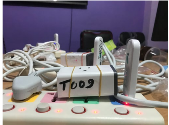
Monitoring electricity consumption of induction stoves with a digital aggregate power meter. Consumption data were transferred over cellular networks using a mobile hotspot device.
