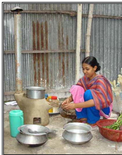
Fig.No.18. Improved Single Mouth Cooking Stove with Chimney (Portable)
