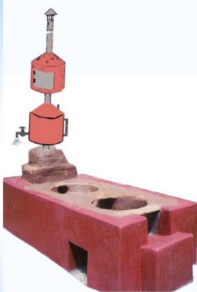
Fig No 29: Improved Double Mouth Cooking Stove with Chimney for Large Scale Cooking Coupled with Water Heater and Oven
