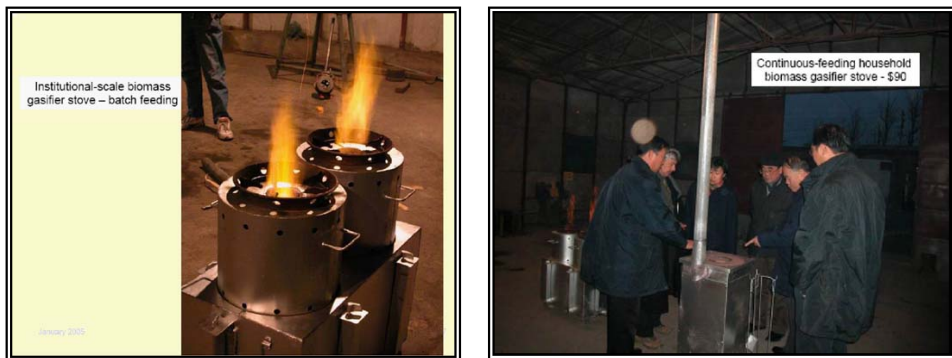
Fig No: 38 Biomass Gasifier Stove for Rural Household in China
