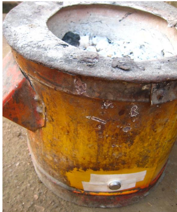
Figure 1: SUMs iButton installed on a charcoal stove in Uganda.
